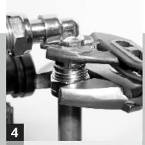
Carefully tighten up the Compression Fitting while securely holding the Angled Service Valve.
