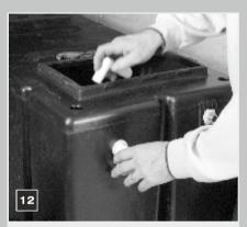
Now assemble the screened elbow filter/mesh warning pipe into the other hole. This warning pipe accepts any 22mm overflow pipe including copper then push fit the dip tube internally into the elbow.
