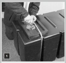
Carefully cut the security straps on the lid/s of the tank.Remove the kit inside the tank and take the contents from the plastic bag.
