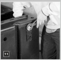
Add the screw and tighten the ball valve fitting. Hand tighten and then tighten with spanner 1/2 a turn. Do not over tighten.
